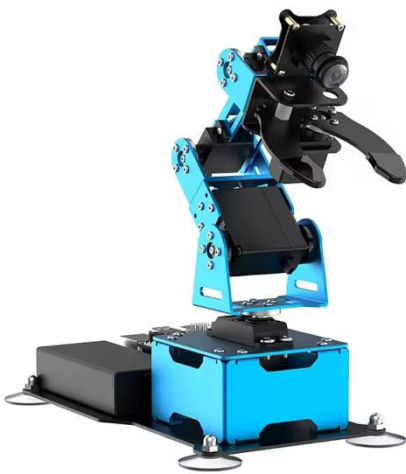
Fig. 4 shows the Hardware implementation of Robot manipulator arm with Raspberry Pi 4 and camera
